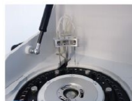
Washing Probe Independent 2-step washing system.
