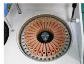
Reagent Tray Refrigerated tray with independent switch.
